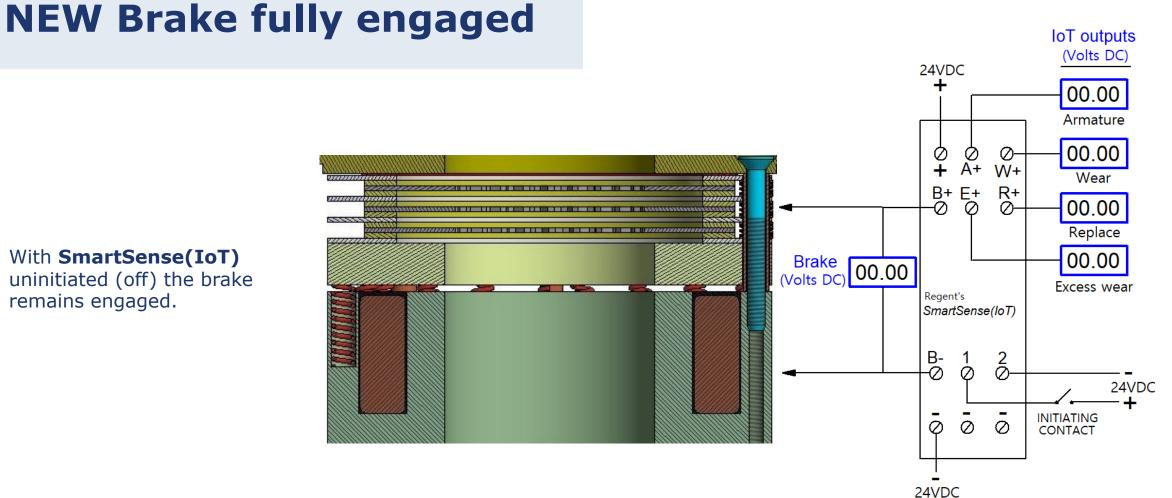
With SmartSense(IoT) uninitiated (off) the brake remains engaged.
